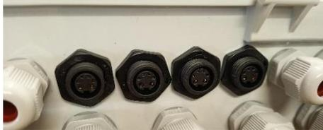
Figure 64 – 4 prises Modbus IP67
